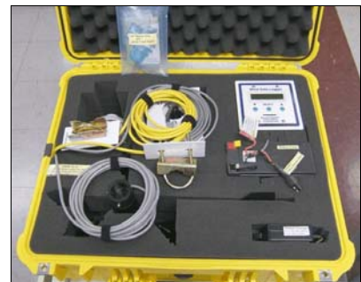
110-WS-25DL-PA or PB Data Logger in Carrying Case with 12V 7AH Battery & AC Charger
