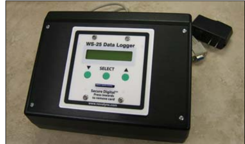
110-WS-25DL-D Desktop Data Logger with Display with AC Power Adapter and Serial Output Cable
