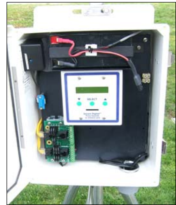
110-WS-25DL-N Data Logger in NEMA Enclosure with 12V 7AH Battery & AC Charger, Surge Protection
