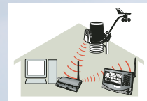
Retransmite de Weather Envoy a la consola
